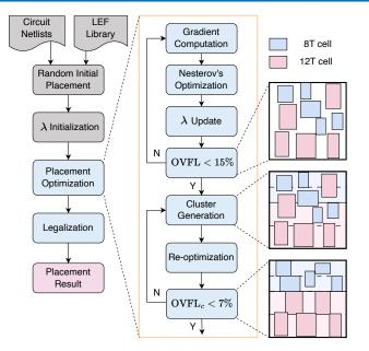
Considering the density constraint for each cell type *c* as a distinct electrostatic system, we frame the placement problem with NIMH cells as follows:
