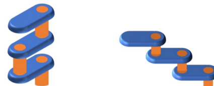
(a) The offset vias that occupy the same region in each layer.
