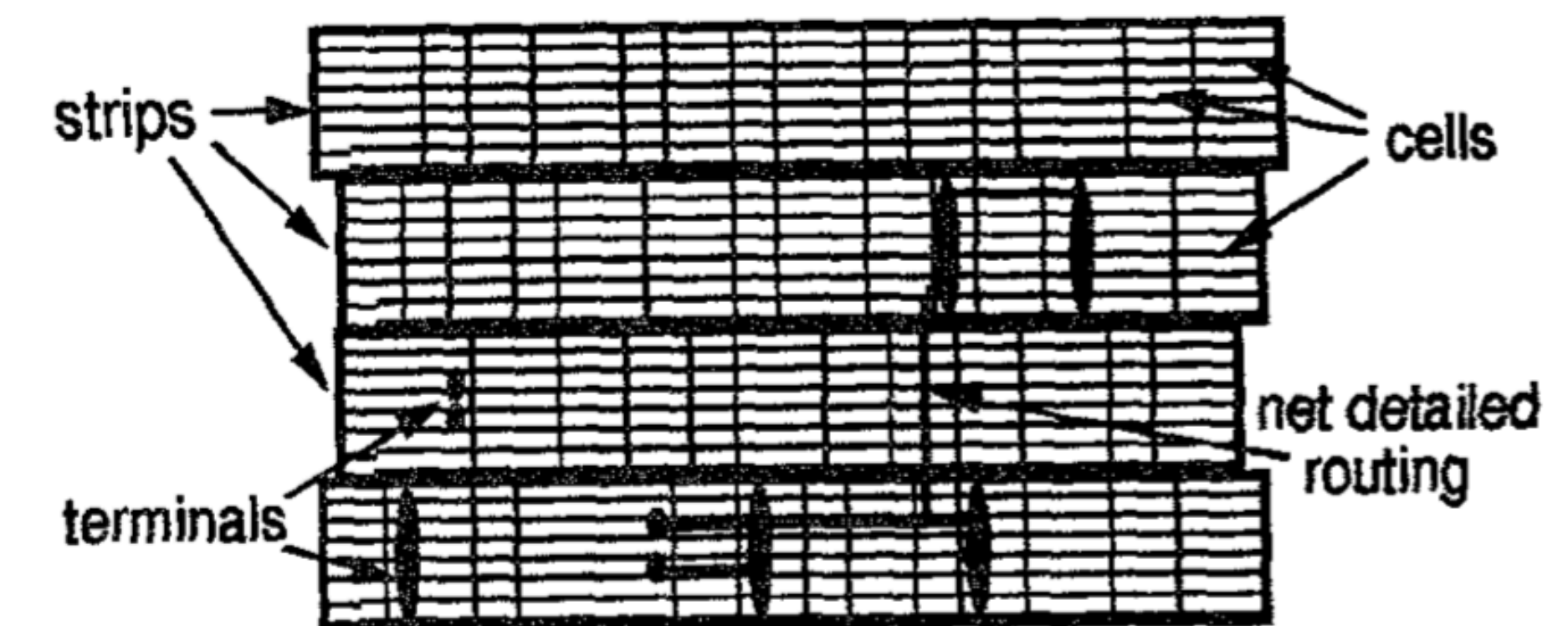
Fig. 3. Transparent Cell circuit structure.
