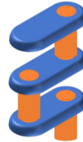
(a) The offset vias that occupy the same region in each layer.
