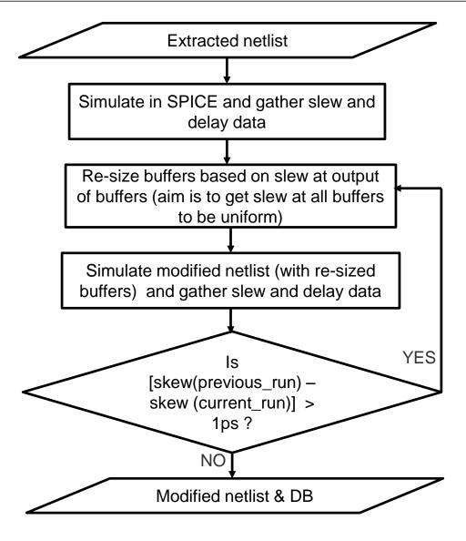
Buffers are sized based on output slew
