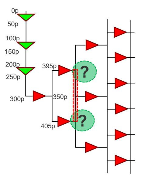
STA cannot handle re-convergence in non-linear circuits.
