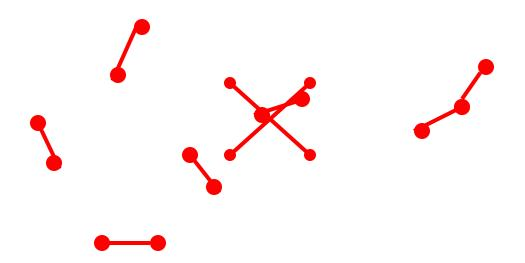
Manhattan Distance: DPL Threshold  $\leq 2\times$  Min Spacing Euclidian Distance: DPL Threshold  $\leq \sqrt{2}\times$  Min Spacing
