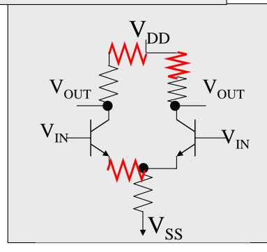
Parasitic elements are generated by cell placement and wiring.
