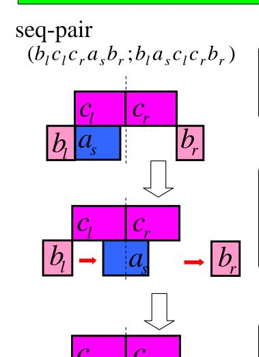
• Cells are packed leftwards based on a given sequence-pair and x coordinate of the axis is determined.
