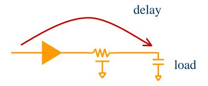
$$r = \frac{\text{delay without interconnect}}{\text{delay with interconnect}}$$
