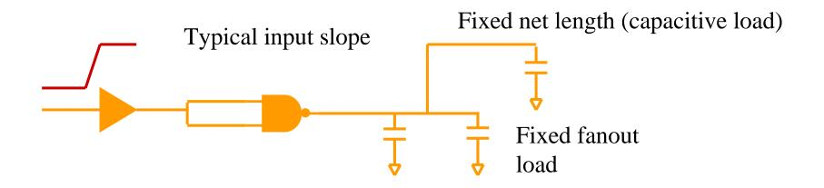
$r = \frac{\text{Fanout delay without interconnect}}{\text{Fanout delay with interconnect}}$
