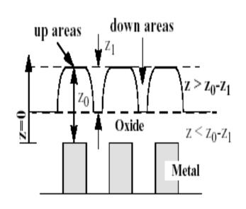
z = final oxide thickness over metal features
