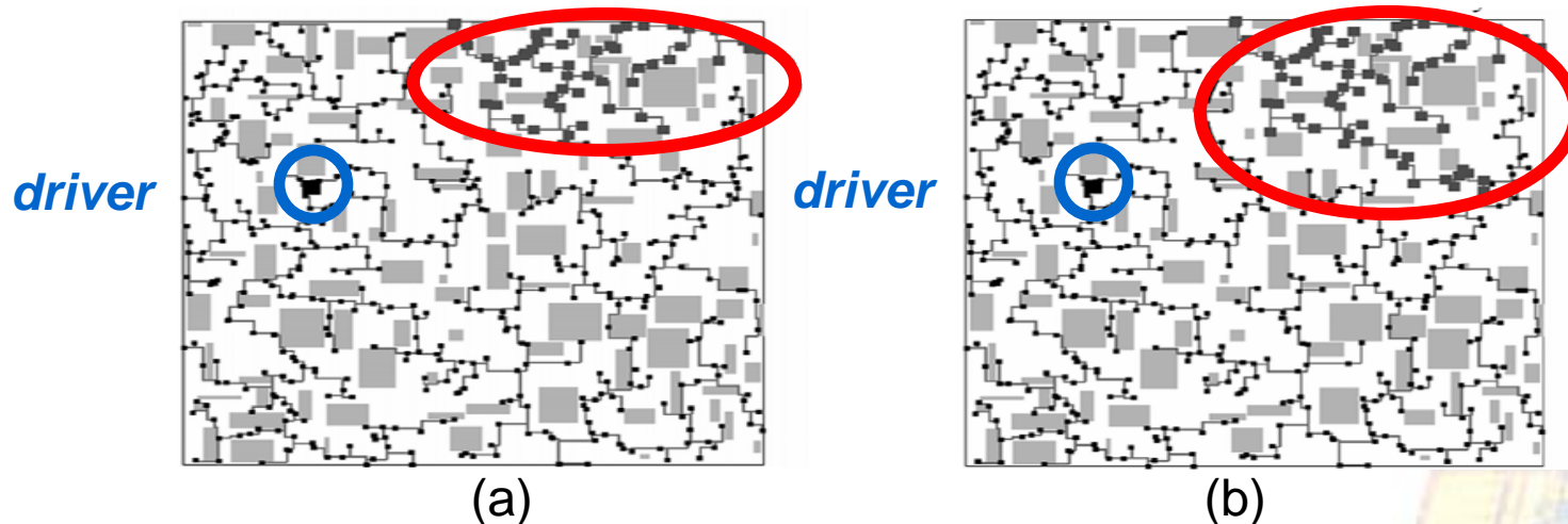
Figure 2. Relation between radius and delay in Minimal Steiner Tree (MST)
